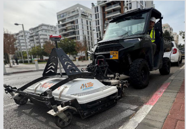
Left: Maya's experts are measuring the surface with the GPR-HDR tool and a base-rover GNSS set up for positioning
